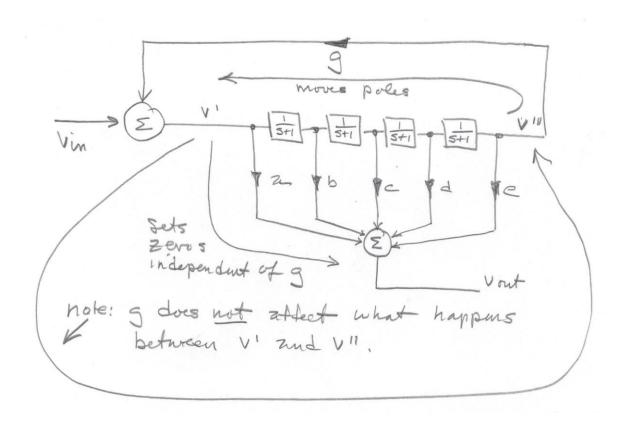
Fig. 1 Four-Pole with Weighted Output
