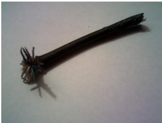
12 conductor cable cut by contractor
