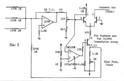
Note: If you need a value of output current different from the current levels developed by the exponential converters in Figs. E and F, connect a resistor to the control voltage summing node and to the positive or negative power supply, for more or less current. Adjust the resistor's value for the proper range.
