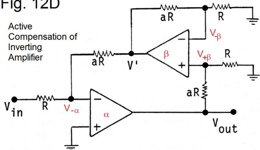
$$V_{+\beta} = \frac{V_{out}}{1+a} \quad (18b)$$
