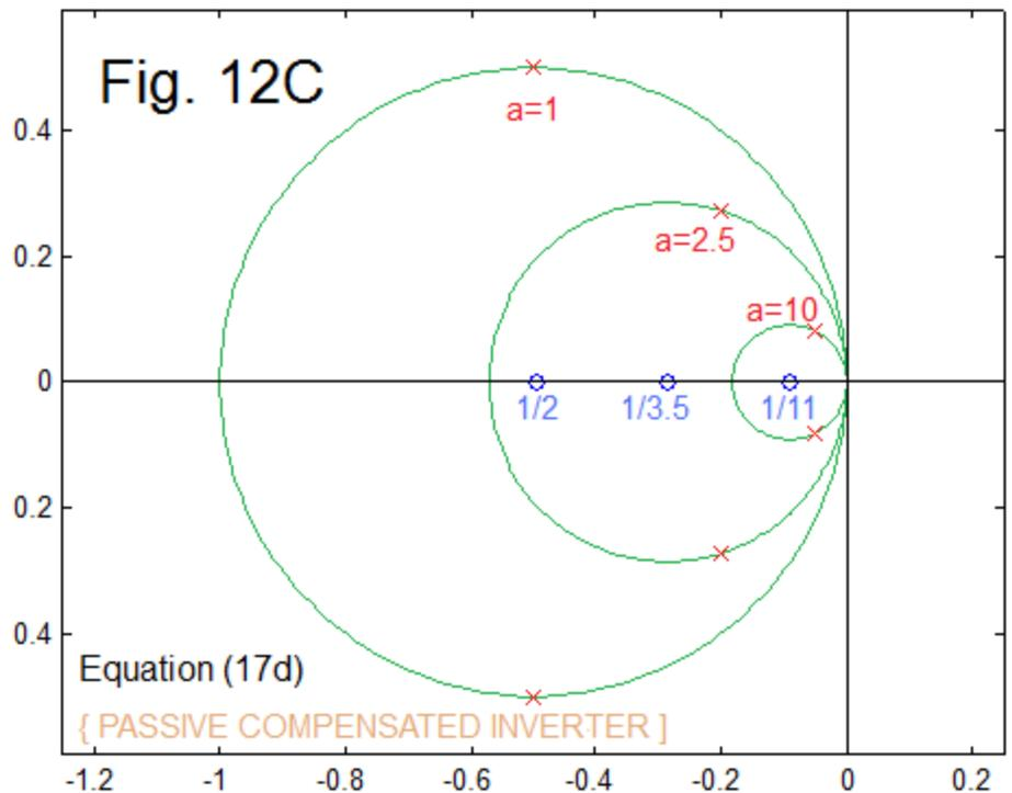
different circles, but always centered on the zero and passing through  $s=0$ , for different values of the gain parameter  $a$ . We show three different cases, for gains of  $a = 1, 2.5,$  and  $10$ . The corresponding zeros are at  $1/(a+1) = 1/2, 1/3.5,$  and  $1/11$ , with the poles on the corresponding circle.
