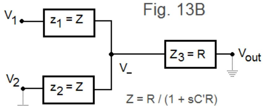
$$V_- = V_1 \frac{[z_2 || z_3]}{z_1 + [z_2 || z_3]} = V_1 \frac{\frac{z_2 z_3}{z_2 + z_3}}{z_1 + \frac{z_2 z_3}{z_2 + z_3}} = V_1 \frac{z_2 z_3}{z_1 z_3 + z_2 z_3 + z_1 z_2} \quad (19a)$$
