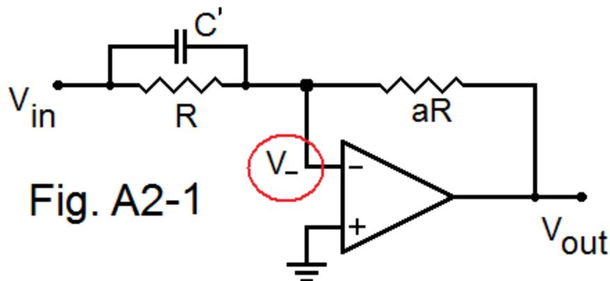
For the moment, we just want to see the effect of the shunt capacitor  $C'$  on the voltage  $V_-$  as it is passed to the inverting input. We recall that the impedance of  $C'$  in parallel with  $R$  is  $R/(1+sC'R)$ . Suppose first that the op-amp is ideal. We have just an ideal inverter, so:
