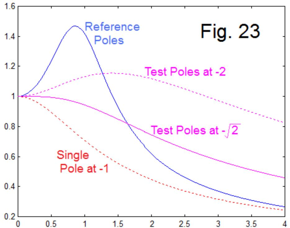
In Fig. 22, we show the zero at  $s=-1$  and “reference poles” at  $s = -\frac{1}{2} \pm \frac{j\sqrt{3}}{2}$  which has been a frequently-observed “magic circle” result which optimizes phase. We notice that the corresponding magnitude response of Fig. 23 has a pronounced bump of nearly 1.5 as we
