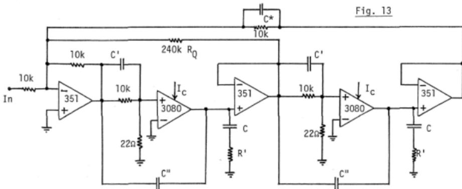
LM351, has a pole at -4.5 MHz, but here it is working at an effective gain of 3, so the pole is moved in by that factor, to -1.5 MHz. Thus  $C^* = 1/2\pi(10k)(1.5\text{MHz})$  is about 10 pfd. [Note that  $C'$ , if set to cancel  $G$  of the integrator op-amps, would be only 3.5 pfd.]
