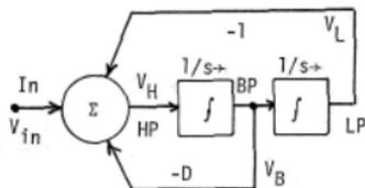
Unlike with many other filter structures, we can often work with a very general model of the state-variable filter and derive performance parameters from the model. We do not always have to do a full analysis with R's, C's, and op-amps. For example, we have related above the equivalence of the Q of the filter to the reciprocal of the feedback path from bandpass to the summer output. Thus, if we can determine this path value, we can get the Q without an analysis of the structure.
