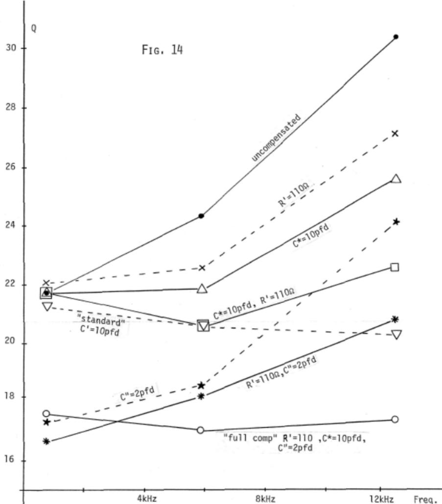
The curves that hover around  $Q = 17$  at the low frequency end all have the OTA compensated by  $C'' = 2\text{pfd}$ . Note that the use of  $C'' = 2\text{pfd}$  only (\*) does not help much, with  $C''$  and  $R'$  being better (★), and the full compensation case ( $R'$ ,  $C^*$ , and  $C''$ , shown by the open circle) is quite good.
