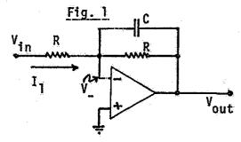
This same current  $I_1$  must be flowing out through the parallel combination of R and C in the feedback loop. The impedance of this loop is:
