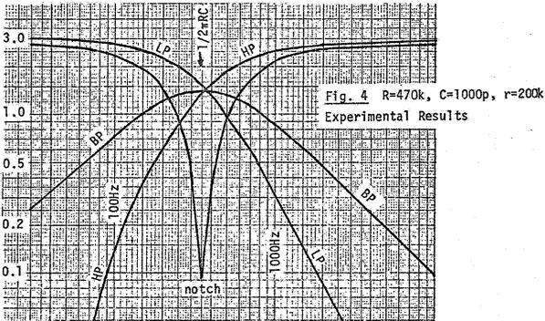
The results in Fig. 4 bear out the theory above. The circuit uses the same number of op-amps as the state variable, except for the notch which uses one less op-amp. The method can be extended to higher order, but component sensitivity becomes more of a problem at third-order, and at fourth-order, resistors and capacitors with a tolerance of 1% are suggested.
