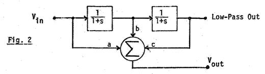
For a weighted sum we have the output  $V_{out} = aV_{in} + bV_{in}/(1+s) + cV_{in}/(1+s)^2$  and we can form the transfer function:
