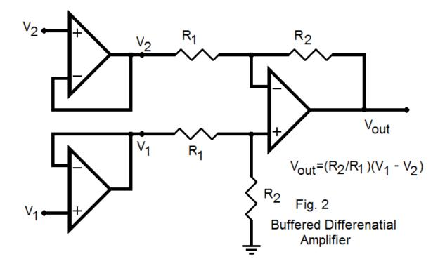
Since the input impedances in Fig. 1 are too low, the use of additional op-amps as buffers (voltage followers) is the next logical step. Fig. 2 shows the two added followers. The equation for the output voltage remains the same.
