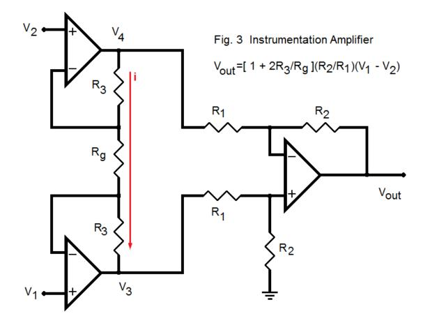
As suggested, there are plenty of ways to make this more complicated than it needs to be. But as with nearly every circuit of practical purpose, there is a "trick" to a much easier solution. Here it is to note that there is a single current i passing through the series resistors  $R_3 \rightarrow R_g \rightarrow R_3$  from  $V_4$
