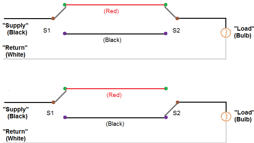
Fig. 2 Two switches (single-pole double-throw) controlling one light - the so-called "three way". Top: one of the two ON states - using the Red wire. By changing S2 (bottom), the light is OFF. Changing S1 will then turn the bulb back on using now the Black wire. And so on.
