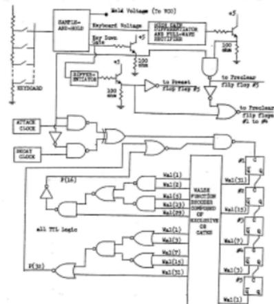
Fig. 7. Envelope controller circuit showing sources of controlling signals and method of obtaining  $P(16)$  and  $P(32)$  from the Walsh functions. The Walsh functions needed for the envelope summer are removed from the decoder.
