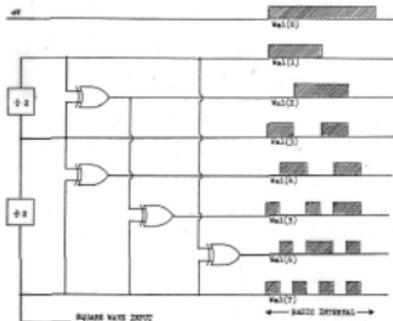
Fig. 1. Digital hardware generation of first eight Walsh functions.
