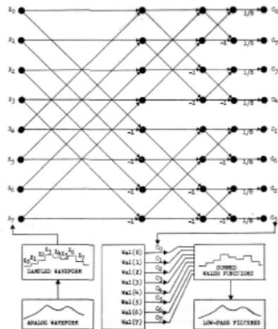
Fig. 3. Overall analysis-synthesis process showing role of Hadamard transform.
